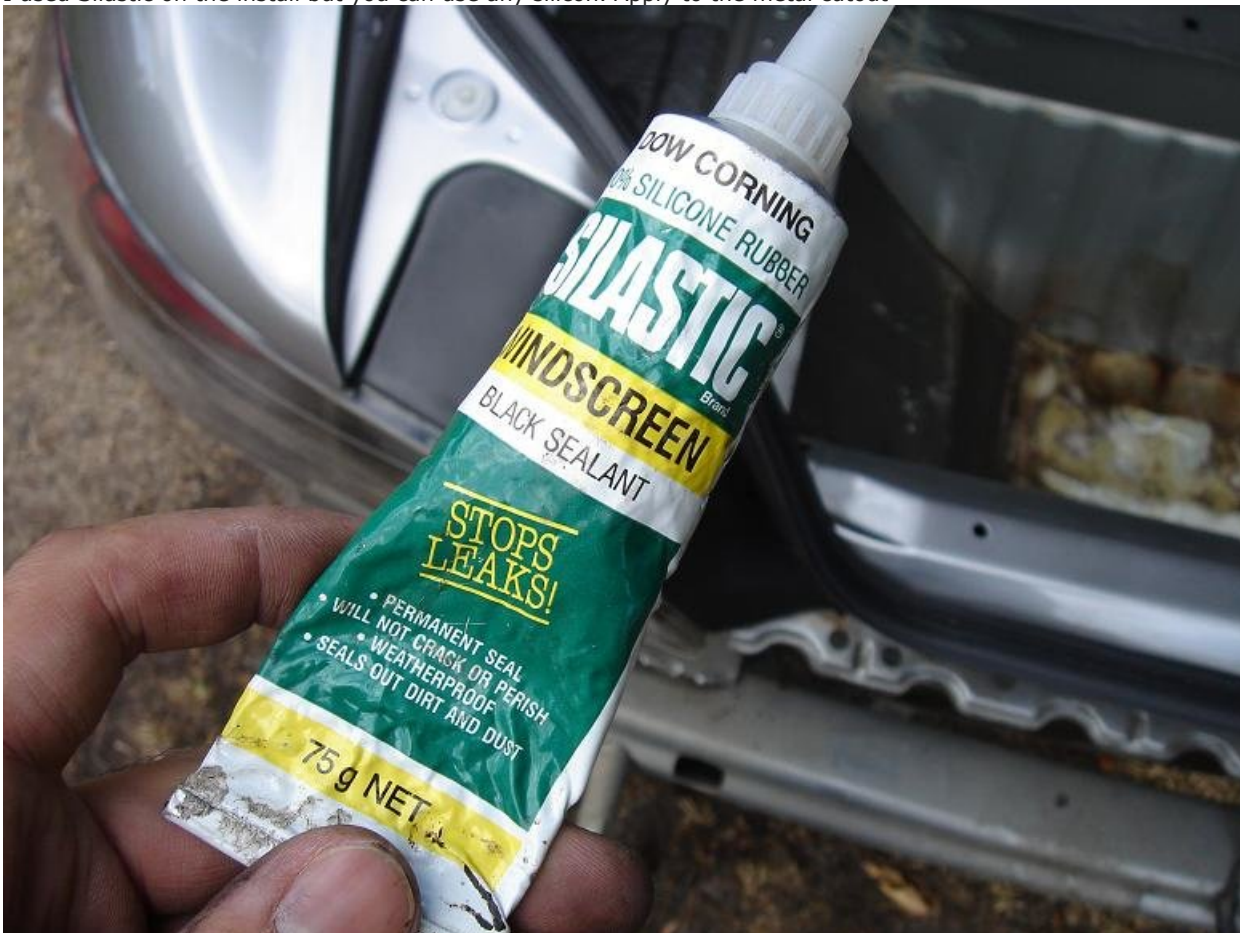
I used Silastic on the install but you can use any silicon. Apply to the metal cutout
