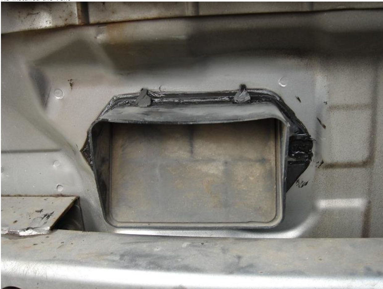
I removed the clips that originally held the vent in as it didn't give the vent a tight fit. I also peeled off the original gasket. Re-installed the Vent
