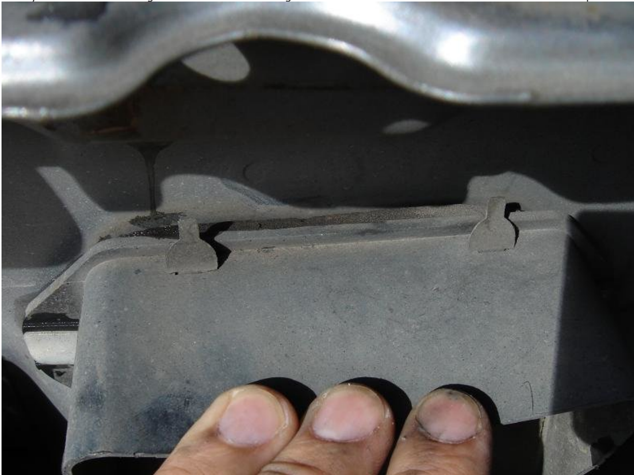
Here you can see that the gasket is worn out making the vent loose. You can also see where the water seeps in..
